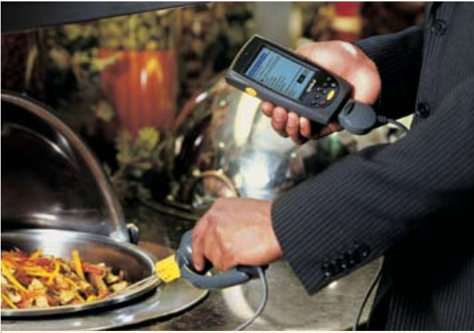
When workers are armed with a mobile computer and a digital temperature probe, employees can quickly and easily monitor food temperatures to protect guest health and comply with government regulations.
